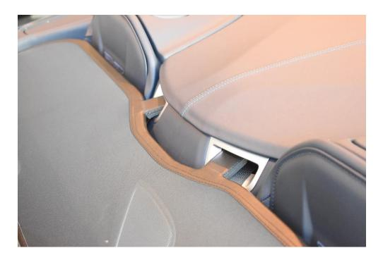
**STEP 3**Unlock the side pins of the wind deflector and click the wind deflector in the factory fitted wind deflector mounts.
