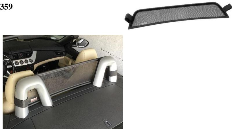
o Open the soft top completely to gain better access to the mounting surface.
